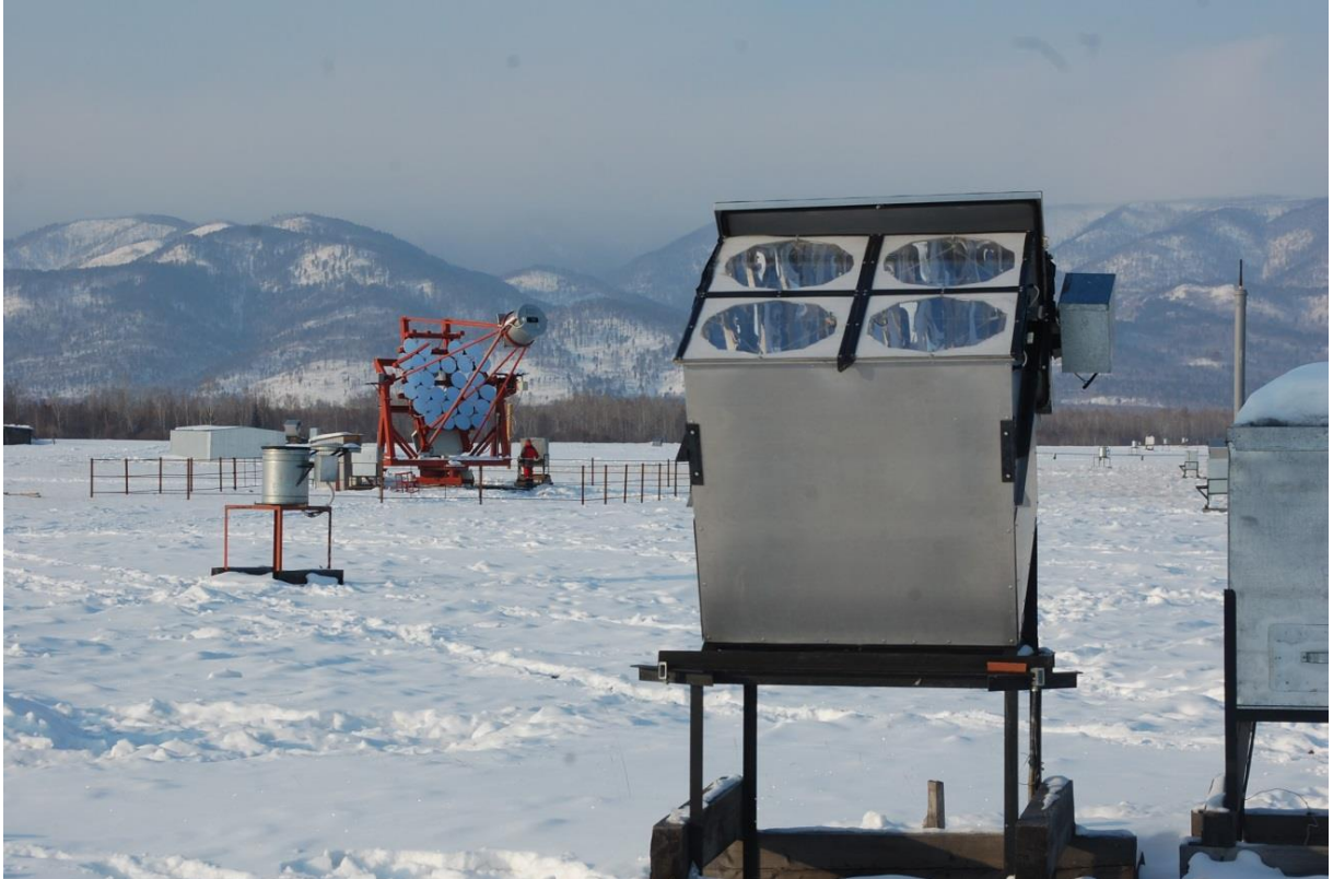
Fig.2. A HiSCORE station with IACT-1 in the background (TAIGA facility in the TUNKA valley, nearby Baikal lake).
